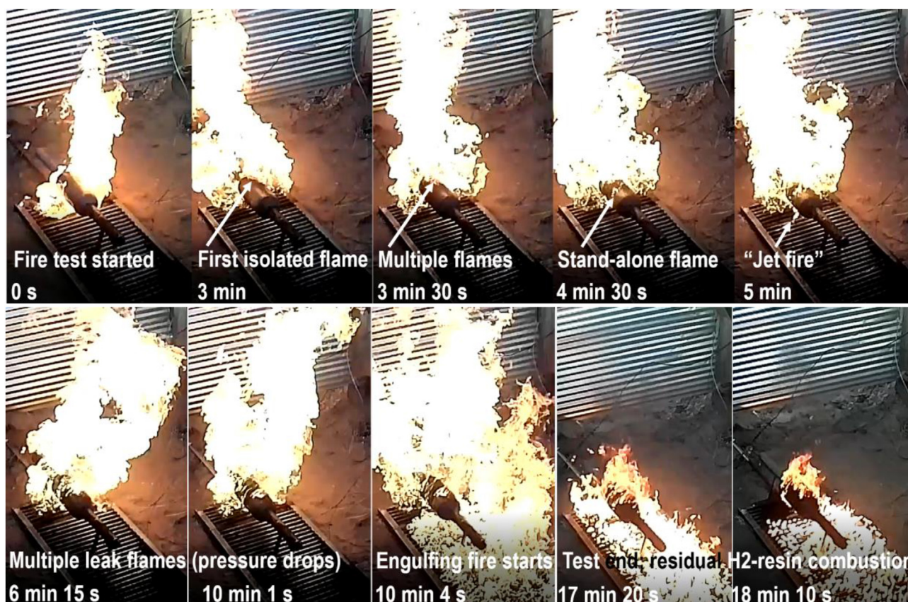
Fig. 5 – Snapshots of \mu LNB tank COPV#CC-4 behaviour in a fire test with HRR/A = 1 \text{ MW/m}^2 .
