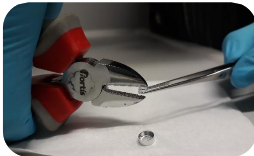
Figure 19. Polystyrene granule sampling for sensitivity test.
