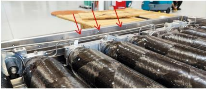
Slightly deformed pipes
