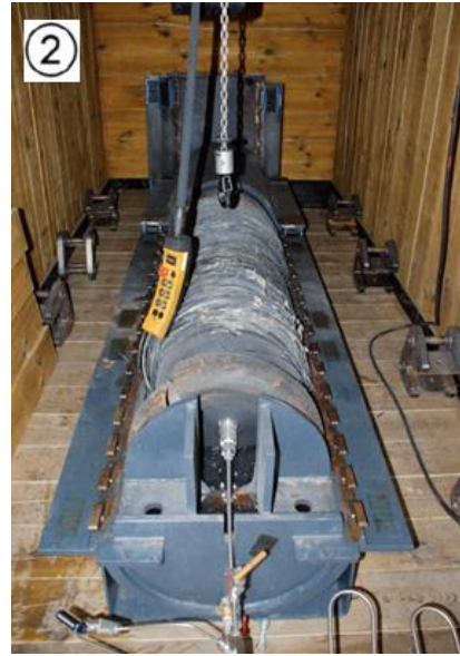
Equipment for hydraulic long-term burst tests
