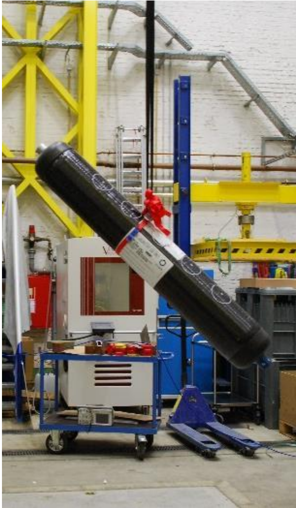
Cylinder drop test
