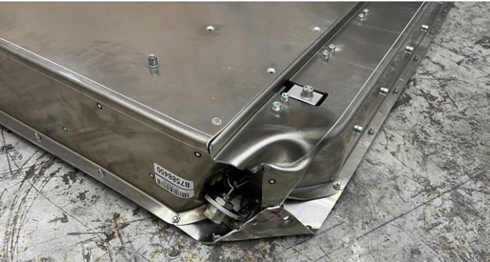
Significant plastic deformation of enclosure
