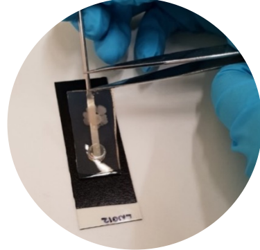
Sample deposition onto an ITO-glass slide
