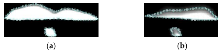
Figure 8. Assigned contours of the cropped ROIs from Figure 7 for calculating the plume area: (a) left direction of view; (b) right direction of view.
