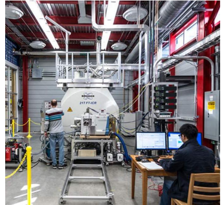
21T FT-ICR MS platform at the NIMFL (2 nd comparable system at PNNL)
