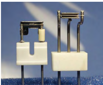
Principle layout of an EI source with photography of filaments
