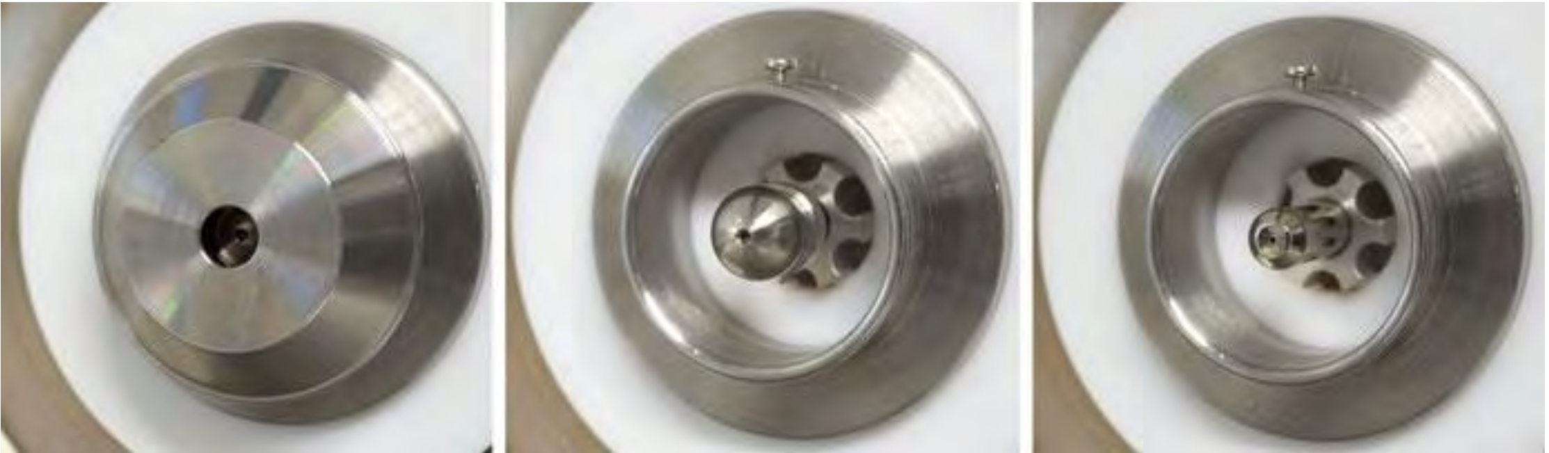
Bruker Apollo II API interface found at almost all Bruker FT-ICR MS
