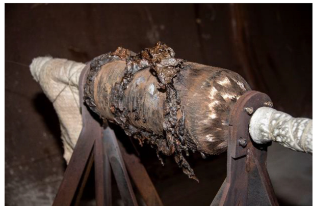
Fig. 7 – Photo of the tank after the impinging hydrogen jet fire test.
