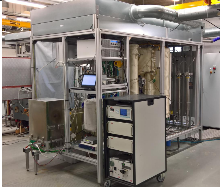
Figure 18 - The INSIGHT test rig for MDLT tool validation located at VTT fuel cell labs.
