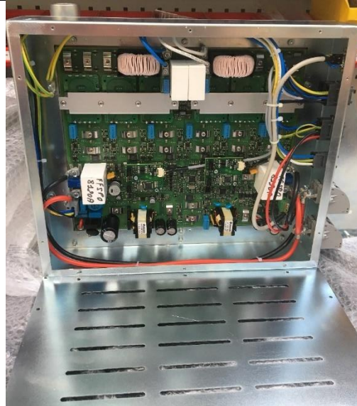
Figure 15 - Modified DC/DC converter for INSIGHT project.
