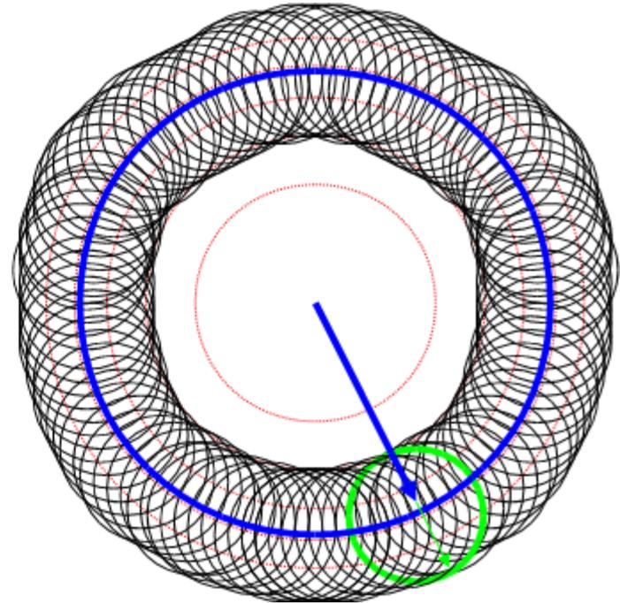
Initial position far from cell center, and low cyclotron motion (ions formed far from cell axis with low initial speed)
