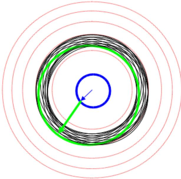
Initial position close to cell center, and cyclotron motion increased (for instance after excitation)
