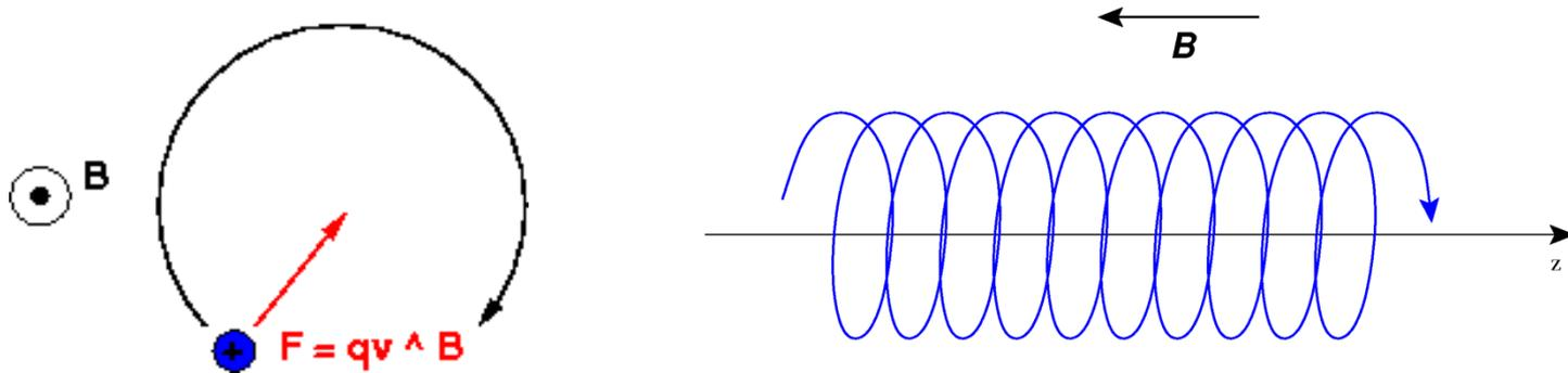
$$\nu_c = \frac{eB}{2\pi(m/z)} = \frac{1.53561 \times 10^7 B}{m/z} \text{ Hz}$$
