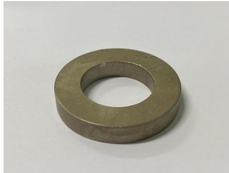
Figure 7. Radial magnet used for the magnetic nozzle
